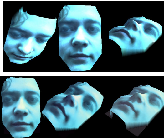
Figure 9 Top: Three views of uncoded face “Image 7”. Bottom, left to right: Coder 3, producing 1.53 BPP at 28.84 MSE, Coder 2, producing 1.35 BPP at 23.76 MSE and Coder J4, producing 1.47 BPP at 25.47 MSE
