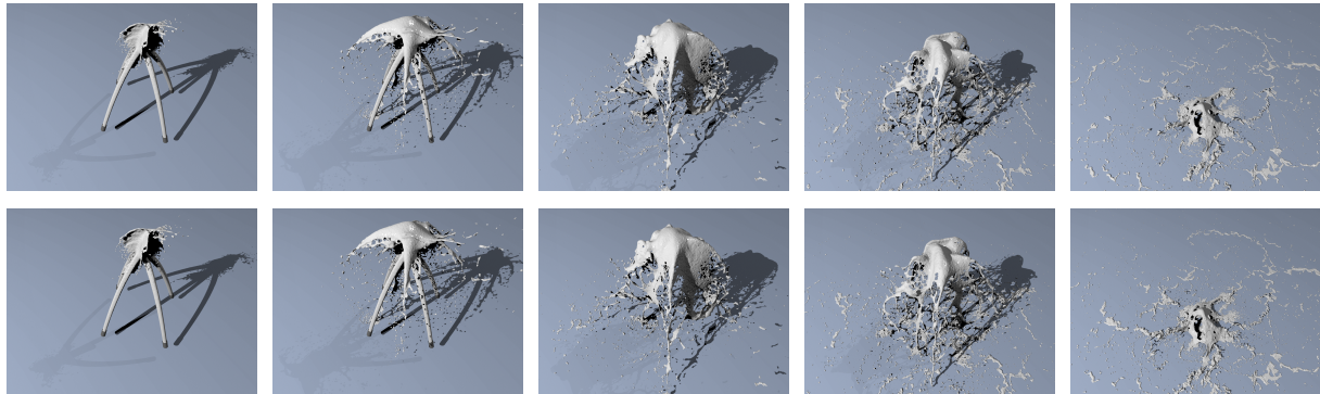
Figure 1: Four jets of liquid simulated with a particle-based simulation. Top: Computed with our GPU implementation. Bottom: The result of the CPU implementation of Chentanez et al. [CMMYK15]. The methods produce similar meshes throughout the simulation. Our parallel self-intersection removal step is 75 times faster and the mesh improvement step 20 times faster than the sequential version. The overall speedup for this example is 50 times.
