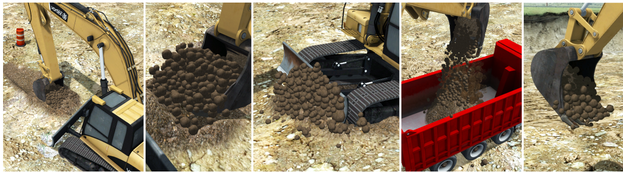
Figure 6: Excavator interacting with a frictional and cohesive loam type soil. Rightmost picture shows adhesive particles stuck to the bucket, which need to be actively released by performing accelerating bucket motions.
