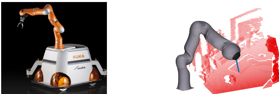
Figure 1: Left: a KUKA Omnirob robot. Right: our scenario: a KUKA robot senses its environment via a Kinect and computes the minimum distance (blue line) to the point cloud.
