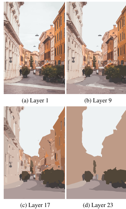
Figure 4: Illustration of the ToS structure. Layer 1 shows a minimally abstracted set of regions, and layer 23 has the highest abstraction with average colors. Original image [Zhy19]
