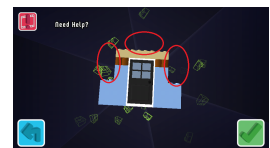
(f) Reconstructed geometry. The red blocks are missing (circled in red).
