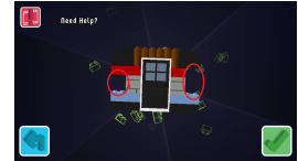
(b) Reconstructed geometry. The white window frames are missing (circled in red).
