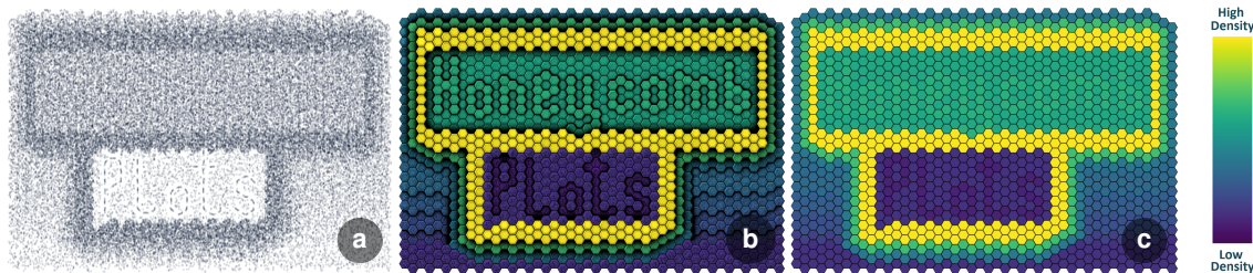
Figure 1: Honeycomb plots (b) combine (a) scatter plots and (c) heat maps using per-tile densities. Through shading, ambient occlusion, and an implicit point-distribution encoding, the observer can explore data features that cannot be captured by either of the techniques alone.
