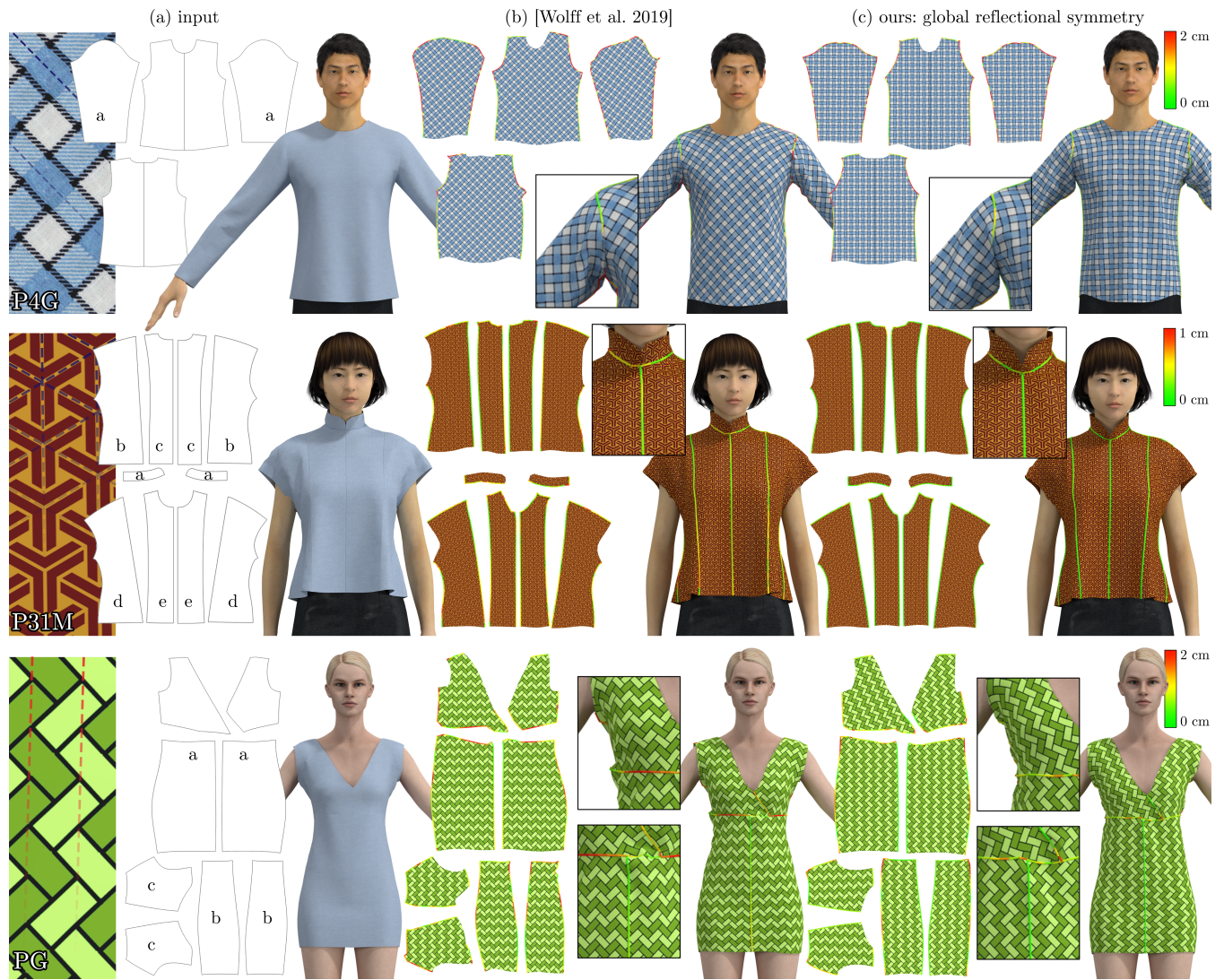
Figure 9: For a given sewing pattern and wallpaper (a), we compare recent work by Wolff and Sorkine-Hornung [WS19] (b) with our altered approach (c). The mismatch d(\mathbf{v}_e) at each seam edge is visualized on a color scale from green (0 cm) to red (2 cm).
