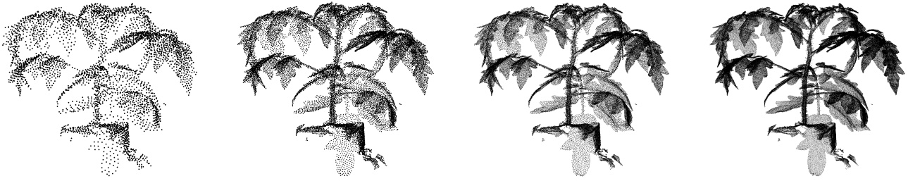
Figure 7: Increasing the resolution from left to right. The resolution levels contain 4.282, 16.499, 59.509, 219.393 points. The scan contains 6.364.517 points in total. Total time: 25.5 seconds.
