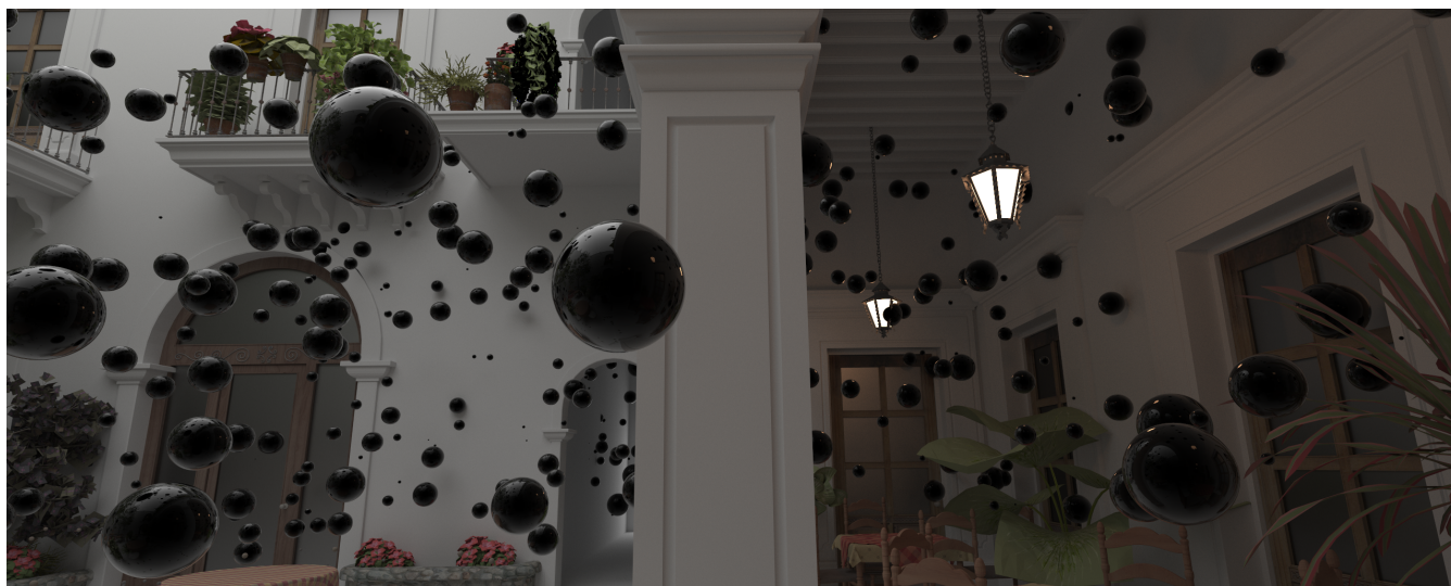
Figure 1: San Miguel triangle scene geometry and reflective spheres rendered using BVHs. We evaluate the throughput of the primitive intersect routine when one BVH is used per primitive type, and when packing triangles and spheres into a single BVH and using compile time polymorphism to determine the primitive type during traversal.
