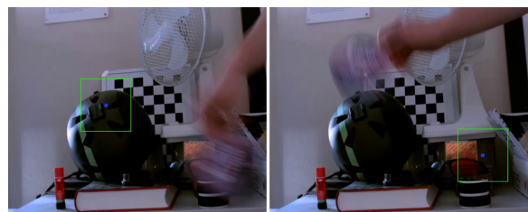
Figure 8: Motion blur is too severe in this scene for feature-based tracking to detect the object.
