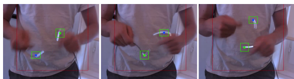
Figure 11: When objects move past each other closely enough, the algorithm is susceptible to confusing them. Here, the green and blue markers switch hands multiple times.
