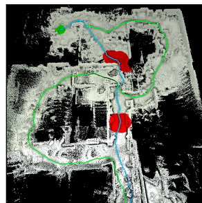
(b) Viable paths through buildings of the Tohoku university with two hazardous environments.
