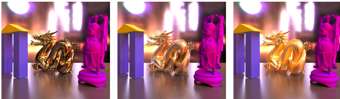
Figure 5: Input image with n = 500 (left); re-shaded dragon surface with n = 10 (center); LuxRender reference image with n = 10 (right). Note that the color saturation in the reference image is also higher due to the fact that the global illumination method accounts for multiple reflections, while in our method a material edit affects one bounce only.
