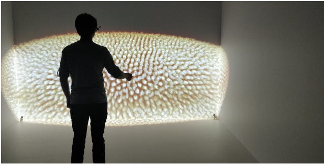
Figure 2: A volume rendering of a developing Drosophila embryo, rendered on a CAVE system. Distributed rendering support is handled by scenery, but not yet exposed in sciview. Image from [GPG*19b].
