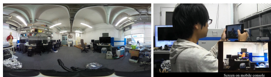
Figure 1: Left: A spherical image; Right: A user controls home appliances using spherical image on a mobile console.
