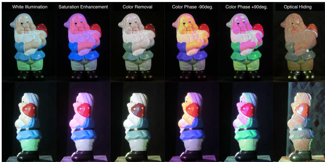
Figure 9: Appearance manipulation results. The top row and bottom row show front and side views, respectively, of the appearance manipulation results obtained using two projector camera units. From left to right, each column shows: the appearance under white illumination, color saturation enhancement, color removal, color phase shift with \phi = -90 degrees and \phi = 90 degrees, and optical hiding.
