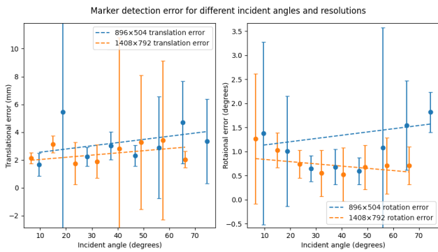
Figure 7: The relation between marker detection error and incident angle. The dashed line represents the linear regression of the error. The incident angle is defined as the combined rotation along the x and z axes.
