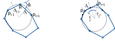
Figure 3: Discrete curvatures: following discrete differential geometry [Bob15] we compute discrete curvatures by considering vertex osculating circles (left), and edge osculating circles (right).
