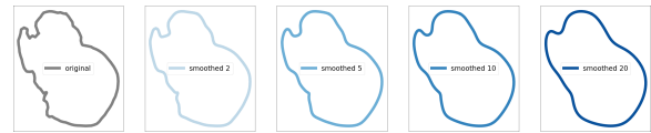
Figure 2: Contour smoothing: we apply iterative contour smoothing to the closed contours (here, N=271 ) extracted from histology images. The higher the number of iteration steps, the smoother the contours: in the example, 2, 5, 10, 20 steps respectively.
