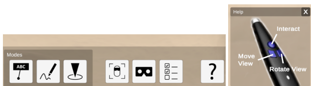
Figure 6: Left: the view-fixed user interface of the semi-immersive teacher system. From left to right: label mode, 3D sketch mode, landmark mode, center view on student, show student's view, show/hide annotations, help. Right: the help menu shows the button layout of the zSpace 's stylus.
