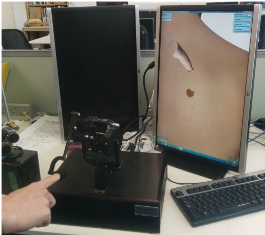
Figure 6: Haptics-based simulator for pigmented skin lesions using a SensAble Premium haptic device.
