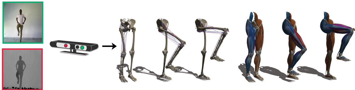
Figure 1: Interactive display of muscle activations during knee flexion. Left: a user moving in front of the Kinect sensor. Middle: activation displayed on action lines. Right: display on 3D meshes.
