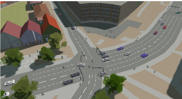
Figure 3: Realistic traffic lanes are generated from OSM data and used for the visualization as well as the traffic simulation.
