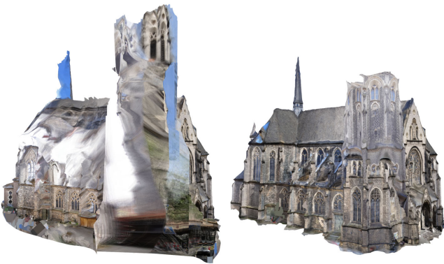
Figure 9: Comparison of a reconstructed mesh before (left) and after (right) post-processing. With our tool, it took less than 10 minutes to obtain the mesh on the right.
