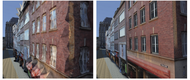
Figure 12: Left: A Poisson-reconstructed building. Right: The same building reconstructed with our procedural approach. The windows have been automatically replaced by a library instance.
