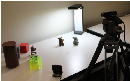
Figure 4: Augmented Reality system setup. The camera on the tripod is used for real time video input and the camera on the table is used to capture environment image for environment map and light source estimation.
