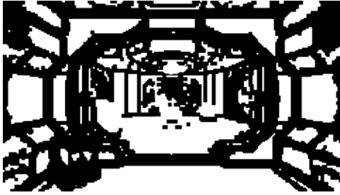
Figure 5: Illustration of culling pre-pass. Areas where no occlusion is estimated are culled (shown in white). Areas that will be calculated in full detail are shown in black.
