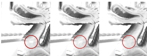
Figure 7: (left) VAO with ‘greedy’ culling pre-pass. Notice white square artifact. (center) ‘Careful’ pre-pass significantly improves result. (right) Reference with no culling pre-pass. Images have been gamma corrected to exaggerate the artifact.
