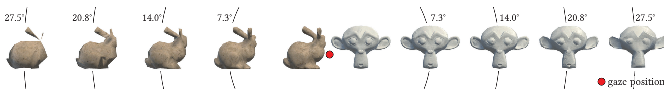
Figure 1: The gaze-contingent perceptual level of detail allows reducing the number of primitives in a mesh in the peripheral vision without impacting the user experience based on viewing parameters. In this figure, we show two example meshes whose geometric complexity is reduced according to the predictions of our method as the meshes approach higher retinal eccentricities relative to the observer's gaze position located at the center.
