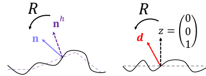
Figure 8: Normal reorientation. We compute the rotation R from the coarse geometry \mathbf{n}^h to the detailed one \mathbf{n} and apply it to a unit vector perpendicular to the plane \mathbf{z} to obtain the detail vector \mathbf{d} .
