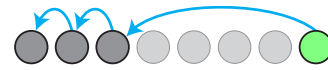
Figure 16: Stateless generation of the 8th y-coordinate of the Sobol' (0,2)-sequence. The coordinates of the 3rd, 2nd, and 1st points are recursively generated.
