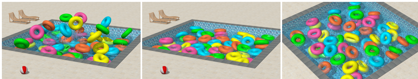
Figure 7: 50 reduced deformable tori (each with 10 modes) fall into a pool ( 256 \times 256 \times 64 fluid grid) and float on water (viewed from two different camera angles). The reduced deformable tori get squeezed and bent as they interact with the fluid and collide with each other.
