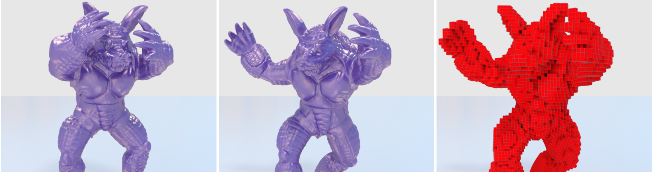
Figure 3: Armadillo model deforming as a result of kinematically animated Dirichlet constraints. Embedding lattice shown on the right.
