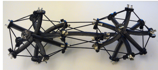
Figure 8: After two weeks, the 3D printed struts have deformed significantly under the tension of the cables.
