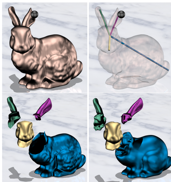
Figure 12: Different representations of the bunny including the articulated skeleton (top right), triangulated surfaces with holes (bottom left) and level sets (bottom right). Note that our algorithm works even with a very crude skeleton. Also note that the skeleton is not perfectly embedded inside the body and pops out near its neck region, which our algorithm robustly handles.
