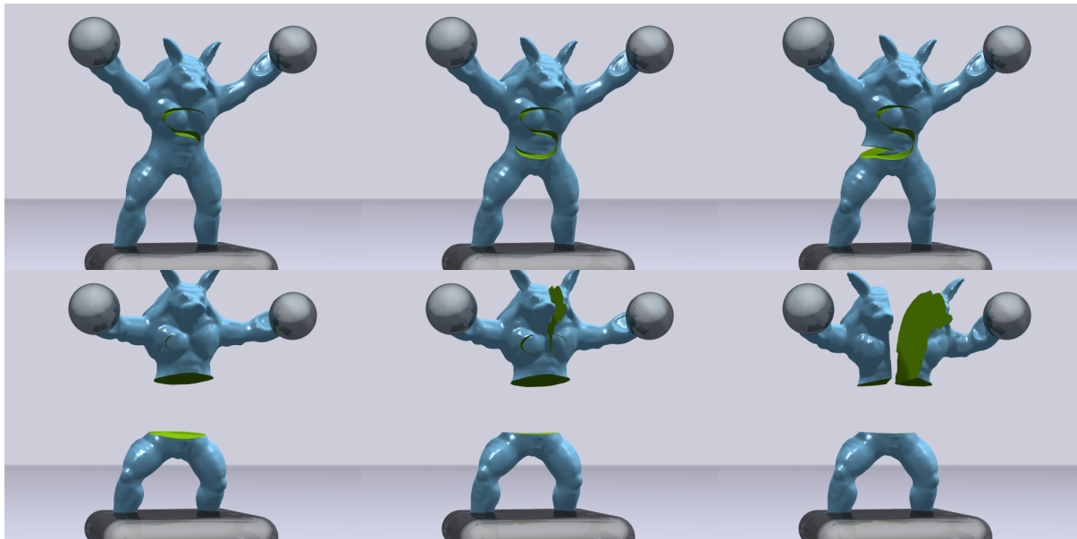
Figure 4: An armadillo mesh with 380K tetrahedra is progressively cut with an “S” and then cut into three pieces.
