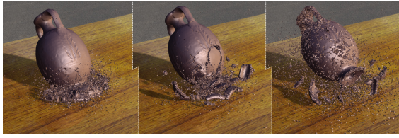
Figure 6: Comparison of vase impact at frame 227 for varying bulk modulus K = 2.94e8, 2.94e9, 8.82e9 Pa from left to right.
