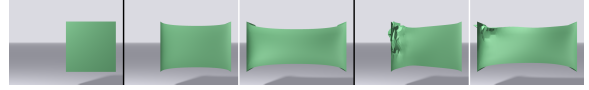
Figure 3: Cube being stretched: initial configuration (left), our method at t = 0.4 s and t = 3.0 s (middle), and standard Newton's method at t = 0.4 s and t = 3.0 s (right). Both simulations were run with one time step per 24Hz frame. Newton's method requires three time steps per frame to converge on this simple example.
