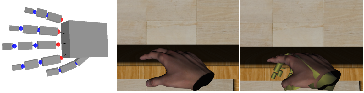
Figure 5: Left: Configuration of the bones and joints that forms the human hand model. Middle: Soft finger contact with a table. Right: Finger contact, showing target configuration tracked with a Cyberglove (in yellow).
