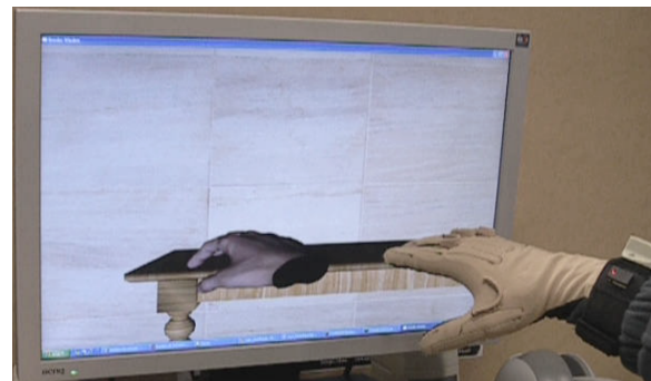
Figure 1: Interactive simulation of a hand with articulated dynamics and soft finger contact. The hand's skeleton follows the motion tracked with a Cyberglove device, and we use our novel algorithm to simulate its dynamics.
