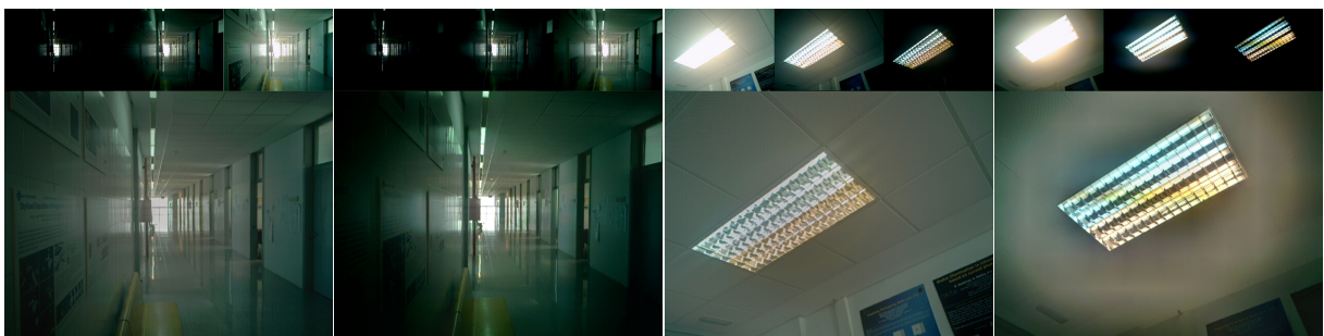
Figure 4: Results obtained with the N900 using our application (left) and HDR Capture app (right) by Nokia Beta Labs. Insets show the images used to build the final one. Examples taken with auto exposure in both applications. We can see how our application produces a more detailed and natural look.
