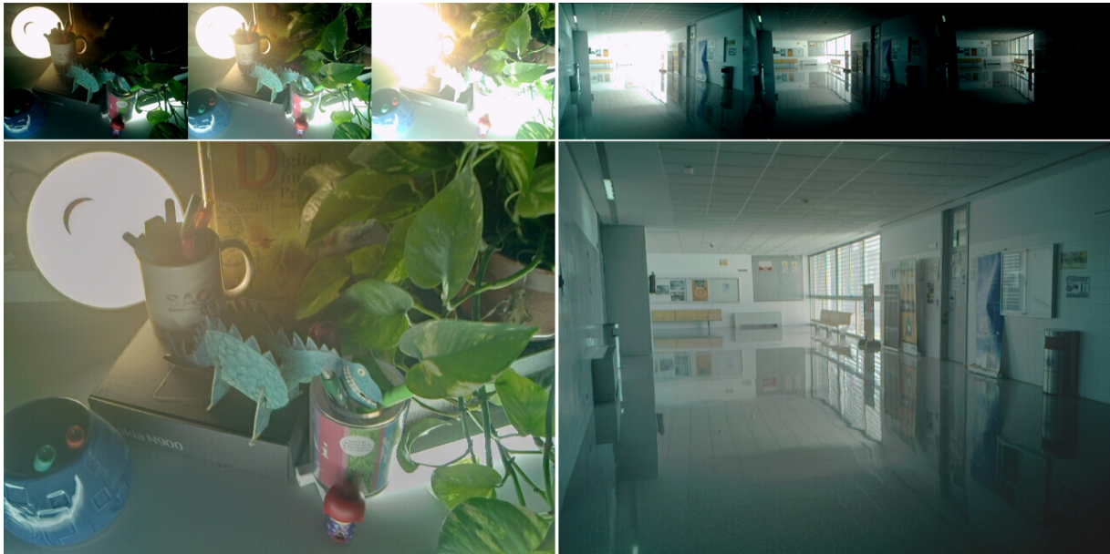
Figure 3: Two examples of photos captured and processed by our method. The insets show the bracketed sequence input. The complete pipeline takes less than 20s for a resolution of 640x480. Left: auto exposure. Right: manual selection of three EVs out of five.
