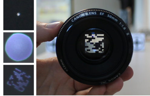
Figure 1: Left: Images of the response to a point light of different apertures (from top to bottom: focused aperture, defocused circular aperture -defocus depth = 90 cm- and one of our coded apertures -defocus depth = 90 cm-, shown in the right). A LED and black cardboard were used to create the point light. Right: Canon EF 50mm f/1.8 lens with one of our coded apertures.
