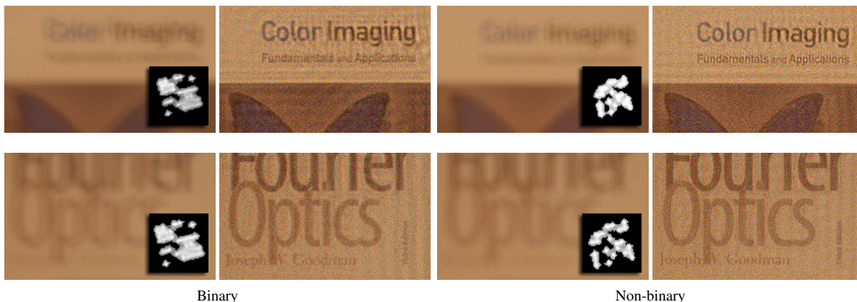
Figure 13: For each pair of images, the left image shows the captured defocused image and the right image the deblurred image. Insets depict the PSF used in each case. Defocus depths are 70 cm (top scene) and 90 cm (bottom scene). The color of the images differs from those in Figure 8; please note that this is due to the fact that illumination conditions during the capture process were different, and not to the coded apertures themselves.
