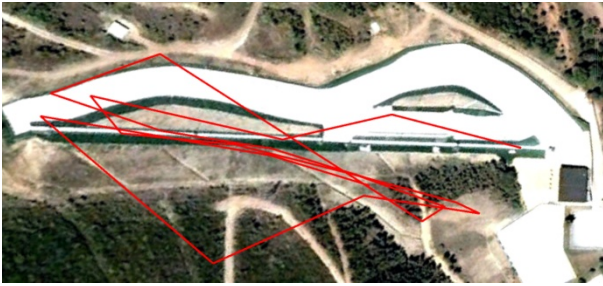
Figure 5: GPS position errors due to an overhead power line and mountain cluttered sky (all locations should have fallen inside the white area).
