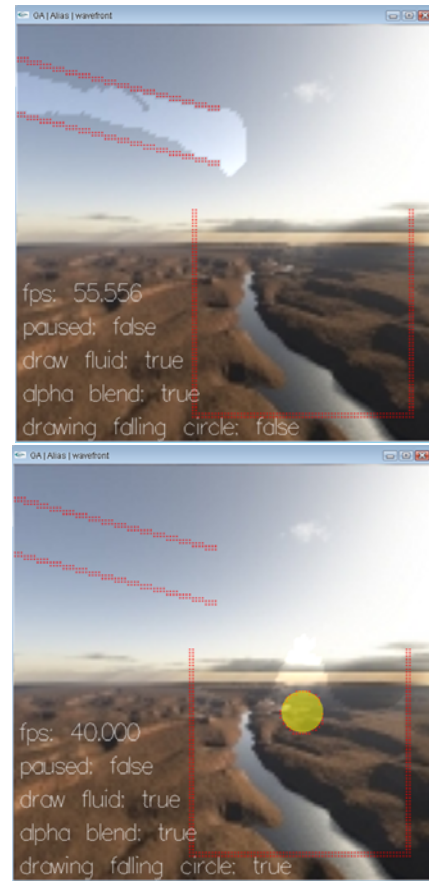
Figure 8. A CPU version of [Stam 03] fluid simulator with internal and moving boundaries (red dots), using the CG solver.
