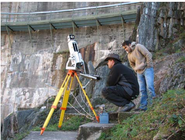
Figure 8: Data acquisition of the Alto Ceira dam, Portugal with a Riegl Z360i coupled with a Nikon D100.
