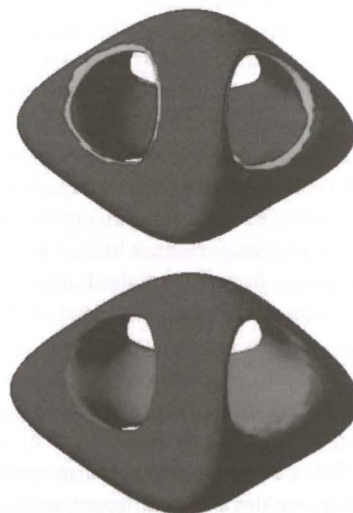
Figure 8. Edge-based segmentation, using k_1 : detected sharp edges (top) and segmented regions for the GENUS3 model (bottom).
