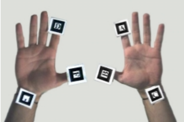
Figure 3: Magic Rings and Magic Bracelets enable the manipulation, through hand and finger gestures, of a filmstrip.
