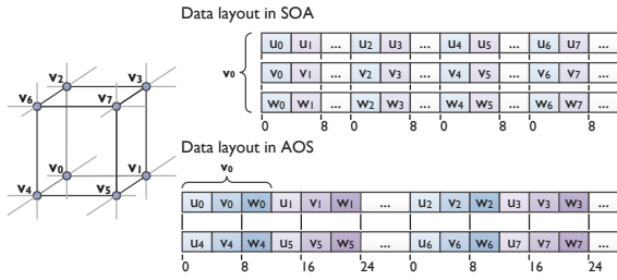
Figure 4: AOS and SOA data layouts for the raw vector data given on a structured grid.
