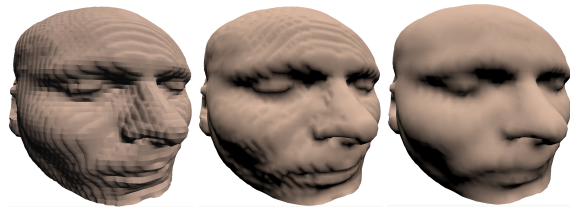
Figure 6: At left artifacts are visible due to sampling error caused by purely local sampling. At center averaging helps but does not remove the artifacts. At right our coarsening removes the artifacts by providing a better local sampling without additional performance costs.
