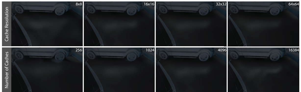
Figure 5: RC resolution and number compared, with a Phong-exponent of 150. If not variable, 4096 RCs at a resolution of 16^2 are used. With low numbers of RCs, details in the reflection are lost, while lowering their resolution makes reflections blocky.
