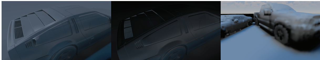
Figure 1: A scene rendered with our method (left). We render indirect illumination (center) using pre-convolved radiance caching (RC); Our contribution is an efficient and robust computation of the RC based on a voxelization (right) and view-adaptive cache placement.
