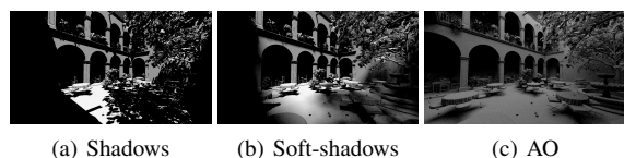
Figure 2: Besides primary rays, we used shadow, soft-shadow and ambient occlusion rays to cover a wide range of ray types. For soft-shadows and ambient occlusion rays, 36 rays per pixel were used. The ambient occlusion ray length is 1/3 of the scene size.
