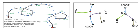
Figure 3: Left: The geometric properties in the feature vector of a branch. Right: Hierarchical decomposition of a rooted tree. Branch B in level one has two children, A and C, each in level two. Branch D, a child of C is in level 3.
