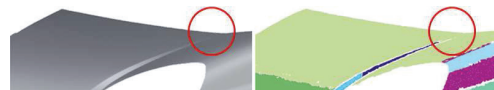
Figure 1: Smoothly connected area and its segmentation: the segmentation was conducted using the method [THH14].
