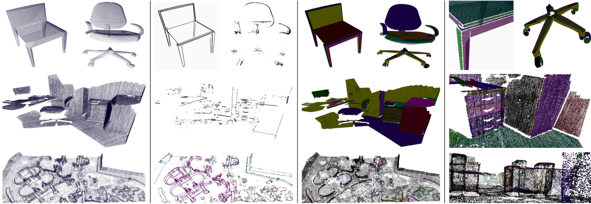
Figure 2: Segmentation process on two separate chairs, office (Nan et al. [NXS12]) and outdoor scene with columns from left to right - all points, edge segments, segmentation results shown as coloured planar segments, close-up view.
