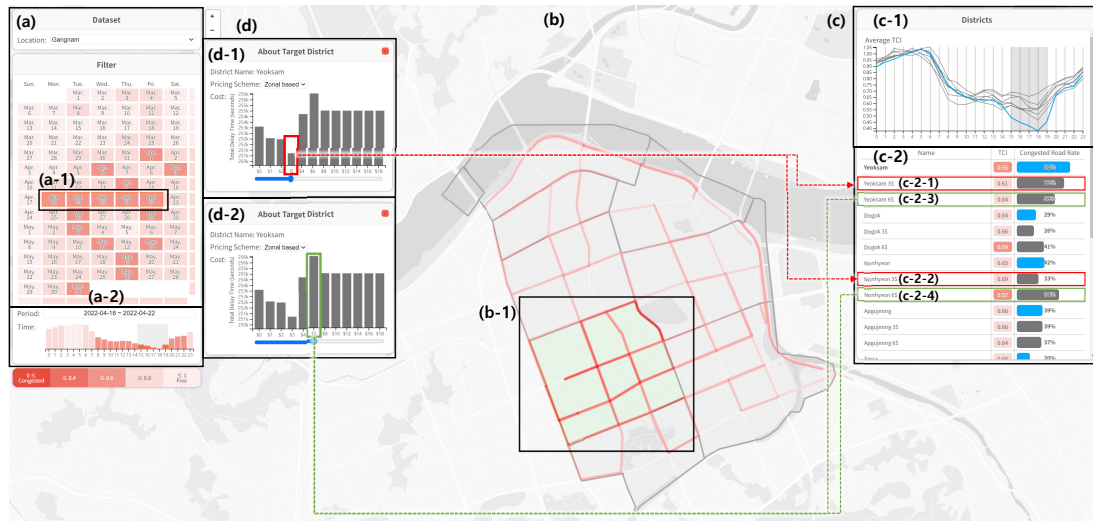
Figure 1: Our system for analyzing the congestion influence of pricing policy. (a) is a filter view for setting the location and time zone. (b) is a map view that visualizes the TCI of the road in the selected time period. (c) is a district view showing the average TCI of roads in each district. (d) is a target district view showing the total delay of the network according to the pricing scheme and toll of the selected district.
